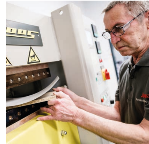
Manfred Palluch uses a press to fix a veneer to a wooden composite design.
