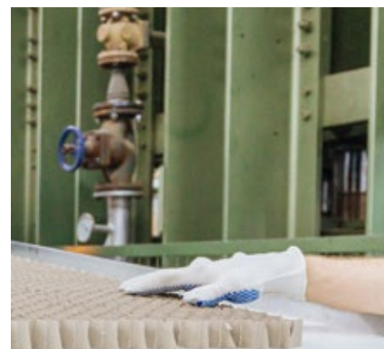
So light and yet so functional: The paper honeycombs are the heart of all VOMO lightweight panels.
