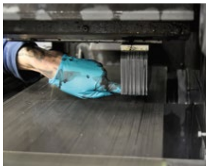
Once the sawing process is complete, the silicon is in slices of around 200 micrometres thick. Source: Fraunhofer CSP
