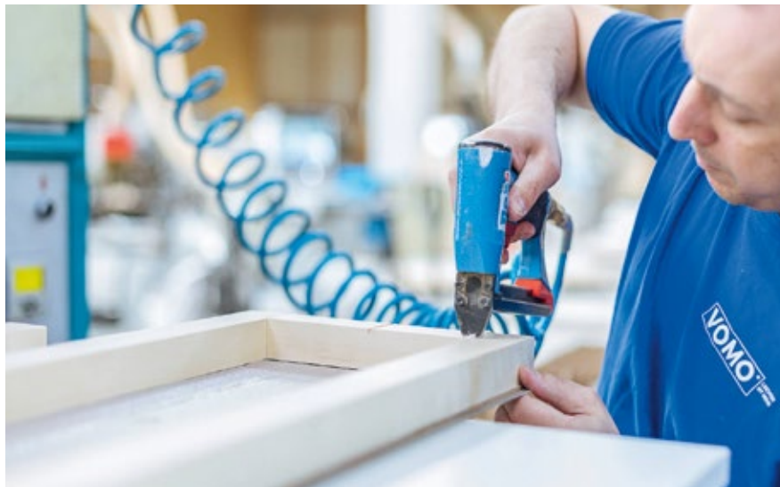
If the lightweight elements are exposed to high loads, a frame made of solid wood or MDF slats gives them additional stability.
